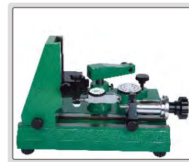
inspect accuracy of test indicators
