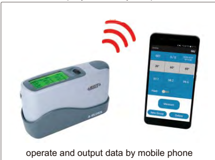
operate and output data by mobile phone
