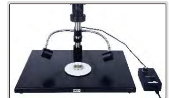
illumination direction and brightness are adjustable
