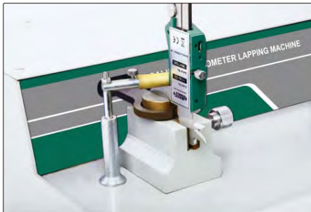
lapping measuring surfaces of caliper lower jaws
